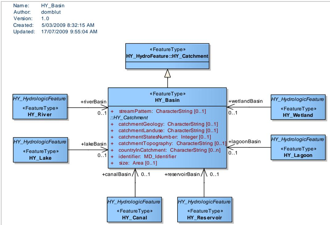
Figure 7 – Basins UML in the GRDC profile
