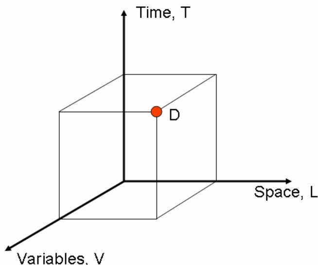
**Figure 5 - The ODM model for hydrological observations**
